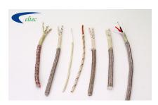
FIBER GLASS WIRES & CABLES are for high temperature applications which has an outstanding and unique combination of electrical, thermal, mechanical & chemical properties. Cable conductors like annealed bare or tinned copper are closely braided with FIBER GLASS Yarn and impregnated with high temperature impregnation.
